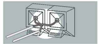
Note: Be Sure to match the speaker cord to the appropriate terminal on the component: + to + and - and -. If the cords are reversed, the sound will be distorted and will lack bass.
